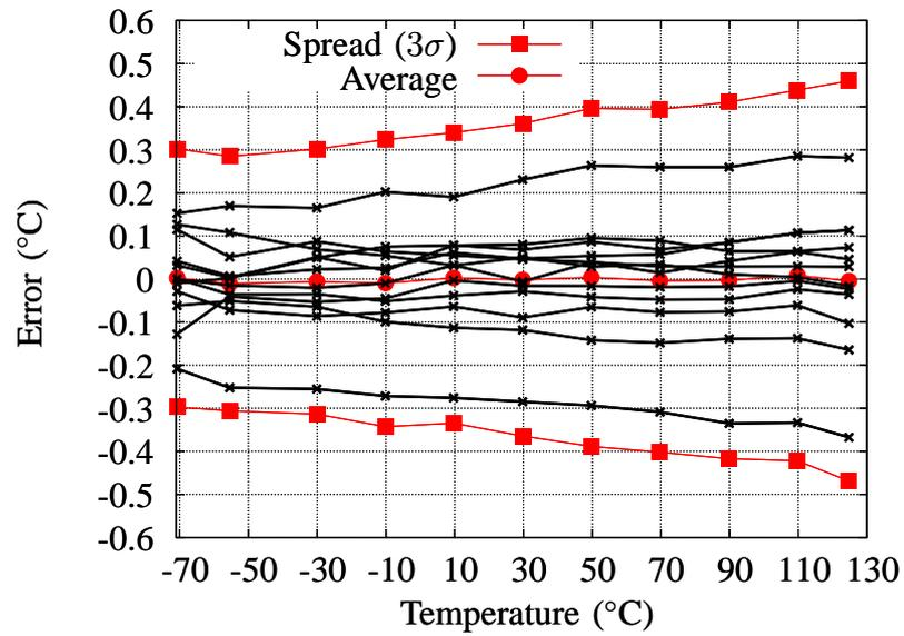
Fig. 14. Measured temperature error (with  $\pm 3\sigma$  limits) of 12 samples after batch calibration.
