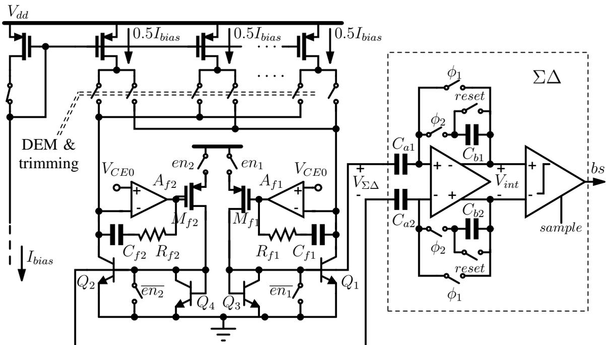
Fig. 11. Schematic of the bipolar core and of the  $\Sigma\Delta$  ADC.
