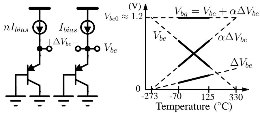
Fig. 1. Principle of operation of the temperature sensor and temperature dependence of voltages in the sensor core.
