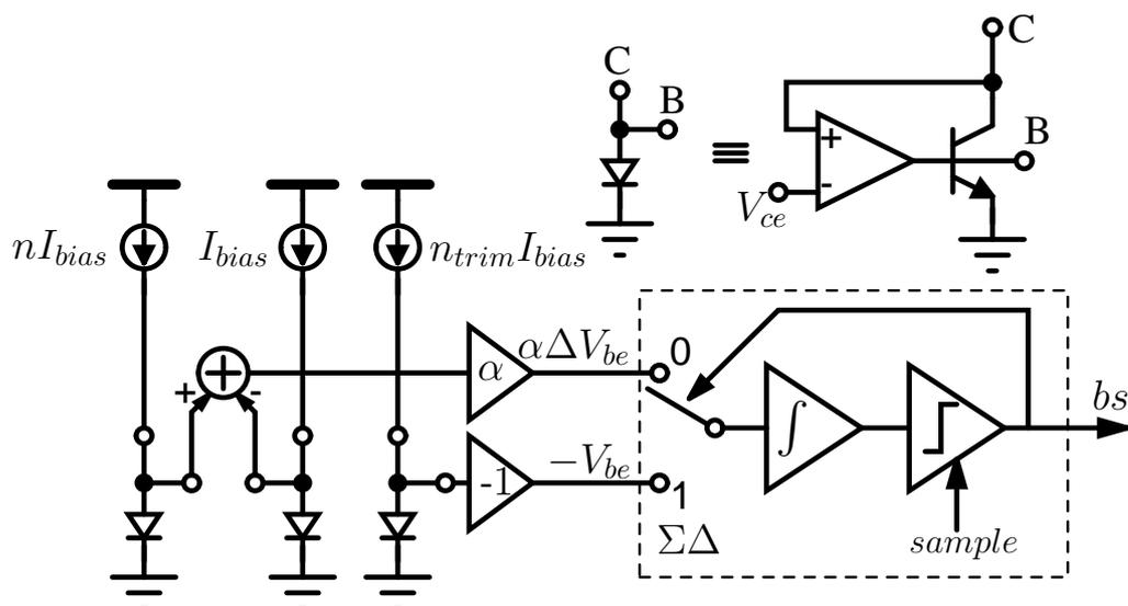
Fig. 5. Principle of operation of the charge-balancing converter.
