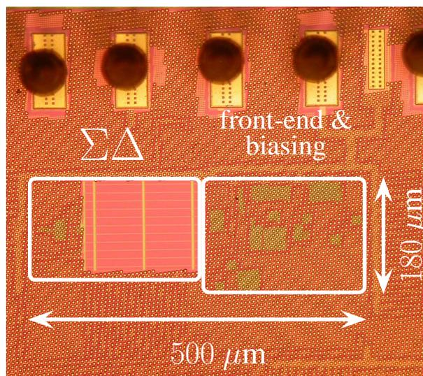
Fig. 13. Chip micrograph.
