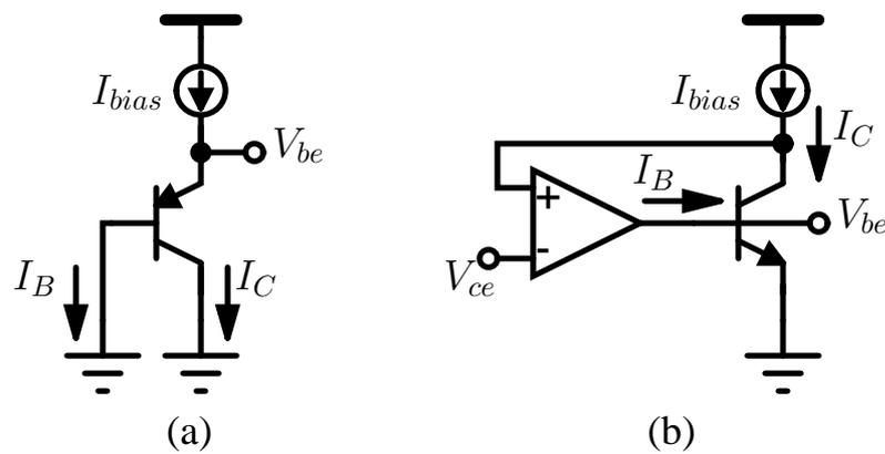
Fig. 3. Bipolar transistors configurations to generate  $V_{be}$  using (a) a substrate PNP and (b) a vertical NPN.
