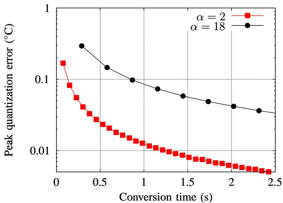
Fig. 7. Simulated peak quantization error over the temperature range from  $-70\text{ }^{\circ}\text{C}$  to  $125\text{ }^{\circ}\text{C}$  versus conversion time for different values of  $\alpha$ .
