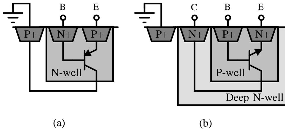
Fig. 2. Simplified cross section of (a) a substrate PNP and (b) a vertical PNP in CMOS technology.
