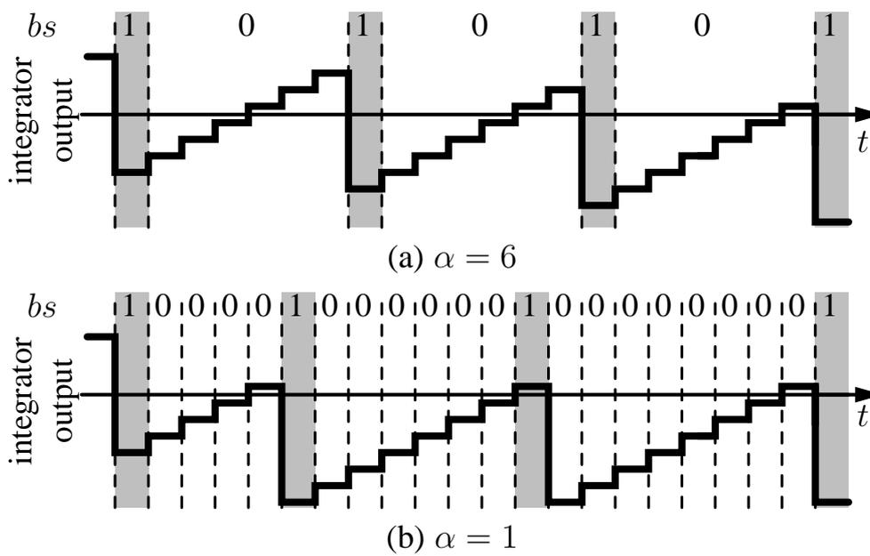
Fig. 6. Integrator output and output bitstream of a fragment of the temperature conversion of the system in Fig. 5 for different values of  $\alpha$ ; the dashed lines indicate the sampling of the comparator.
