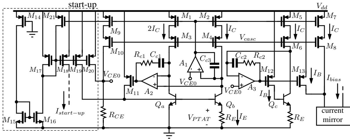
Fig. 10. Schematic of the bias circuit.
