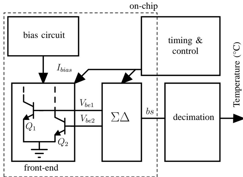
Fig. 8. Block diagram of the temperature sensor.
