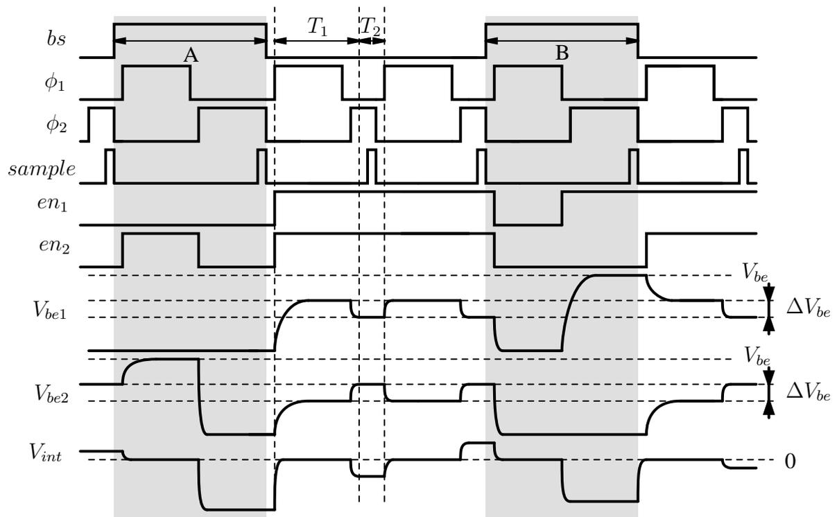
Fig. 12. Timing diagram and waveforms of a fragment of the temperature conversion; periods when  $bs=1$  are shown in gray (A and B).
