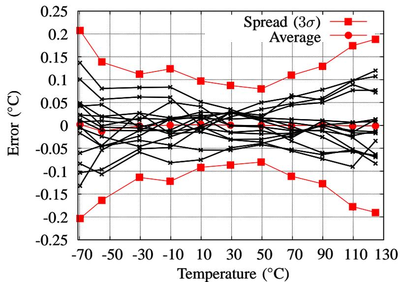
Fig. 15. Measured temperature error (with  $\pm 3\sigma$  limits) of 16 samples after trimming at 30°C.
