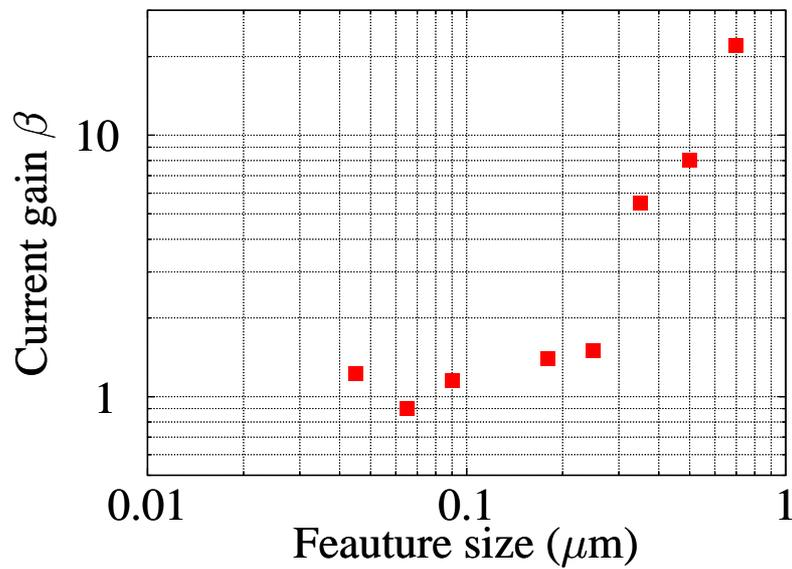
Fig. 4. Current gain  $\beta$  of substrate PNP transistors versus the minimum gate length for various CMOS processes (data from [16] and several design manuals).
