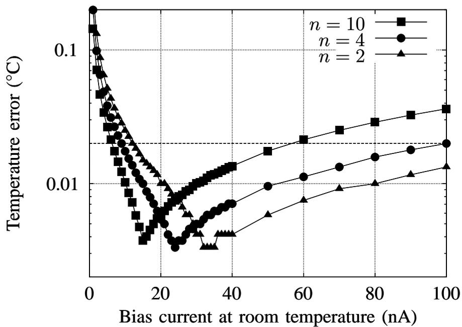
Fig. 9. Maximum temperature error over the military range due to spread in  $\Delta V_{be}$  for different bias current and bias currents ratio  $n$ .
