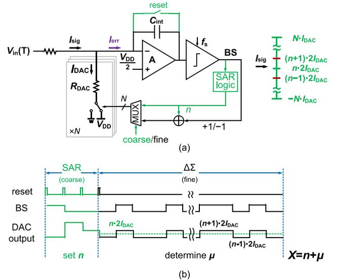
Fig. 6. (a) Schematic of a static zoom CT $\Delta\Sigma$ M and (b) timing diagram example in case of a 3-bit DAC.
