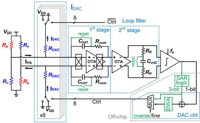
Fig. 7. Circuit diagram of the zoom CTΔΣM.
