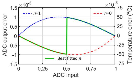
Fig. 11. Temperature error jump when changing  $n$ .
