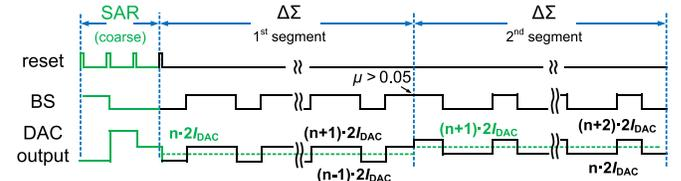
Fig. 13. Modified timing diagram of the zoom CT $\Delta\Sigma$ M.
