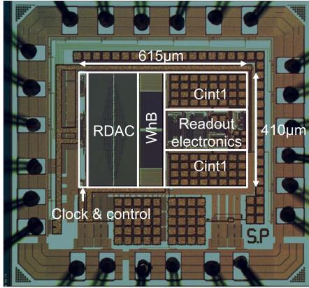
Fig. 14. Die micrograph of the prototype chip.
