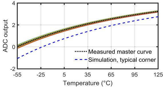
Fig. 15. Measured and simulated sensor output versus temperature.
