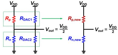
Fig. 3. Balanced WhB with  $R_{\text{DAC}}$  split and merged.
