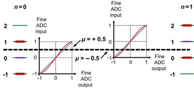
Fig. 10. Readout error of the opposite sign with two possible coarse codes.
