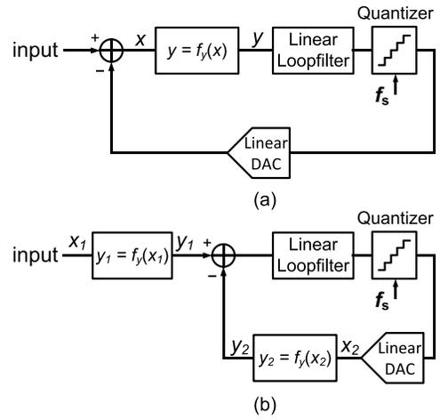
Fig. 5. (a) Nonlinearity modeling of the zoom CT $\Delta\Sigma$ M. (b) Equivalent model of (a).
