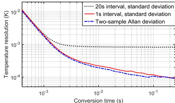
Fig. 21. Temperature resolution versus conversion time using different calculation methods.
