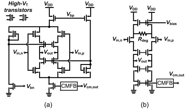
Fig. 8. Schematic of (a) current-reuse OTA in the first integrator and (b) source-degenerated OTA in the second stage.
