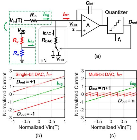
Fig. 4. (a) CT $\Delta\Sigma$ M based on an active integrator. (b) Error current of a single-bit CT $\Delta\Sigma$ M. (c) Error current of a multi-bit CT $\Delta\Sigma$ M.
