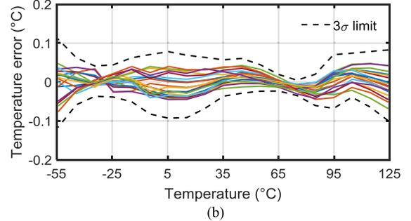
Fig. 17. Temperature error after individual first-order fit and systematic nonlinearity removal (a) without segment averaging and (b) with segment averaging.
