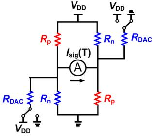
Fig. 1. WhB sensor and DAC using current readout.
