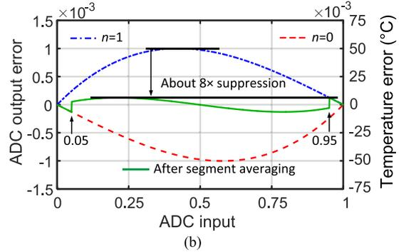
Fig. 12. Nonlinearity suppression using segment averaging (a) without a threshold (b) with a threshold of 0.05.
